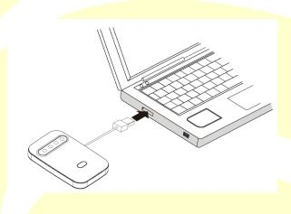
Scenario 3: Multi-device wireless and wired Internet access using Wi-Fi and USB port
