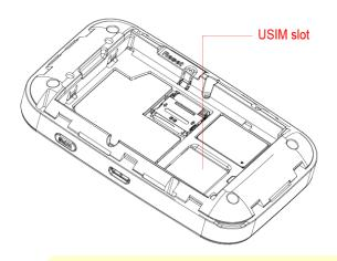
**Note:** Do not remove the SIM Card when the device is on. Otherwise, the card and device may get damaged.
