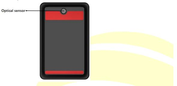
The TMX07 has a built-in optical sensor(optional). When the device is removed after installation and the sensor is exposed to light, it will be activated immediately and the TMX07 will send a "DEVICE\_REMOVED" alarm message to the Platform, together with the current location data.
