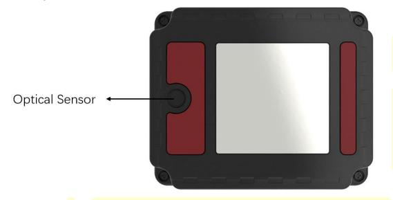
The TMX09-M has a built-in optical sensor. When the device is removed after installation and the sensor is exposed to light, it will be activated immediately and the TMX09-M will send a "DEVICE\_REMOVED" alarm message to the Platform, together with the current location data.
