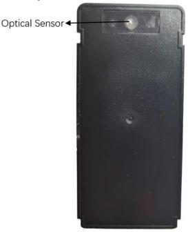
The TMY02 has a built-in optical sensor. When the device is removed after installation and the sensor is exposed to light, it will be activated immediately and the TMY02 will send a "DEVICE\_REMOVED" alarm message to the Platform, together with the current location data.
